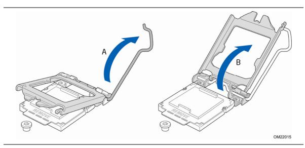
Figure 7. Lift the Load Plate
